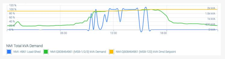
To ensure peak demand is maintained, the Platform monitors kVA demand and increases the BMS load-shed signal if it approaches the setpoint.
