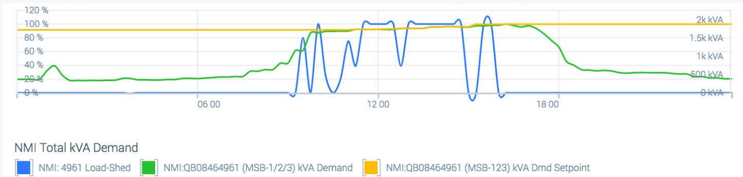
To ensure peak demand is maintained, the Platform monitors kVA demand and increases the BMS load-shed signal if it approaches the setpoint.
